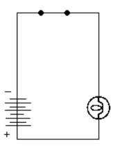
This is an example of a circuit diagram. This circuit has a battery, a lightbulb, and a switch. The switch is closed. This will allow the electrons to flow and the lightbulb will be on.
